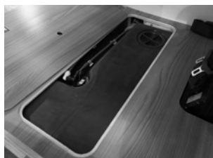
Edge fresh water tank showing central cleaning hatch
