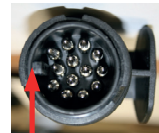
Incorrect alignment Fig. 7
