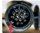
Incorrect alignment Fig. 6
