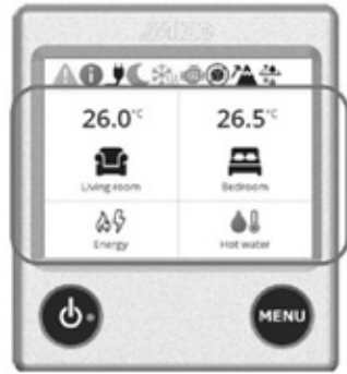
Control panel main menu screen
