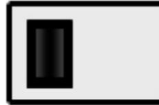
3. Press black isolator button on front of powersupply unit to turn system on. (Button in)
