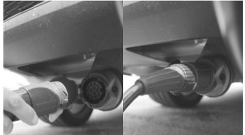
Insert & twist road lighting connector (13 pin plug)
