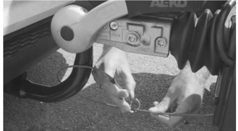
Align the 13 pin plug with the receiving socket on the tow vehicle.
